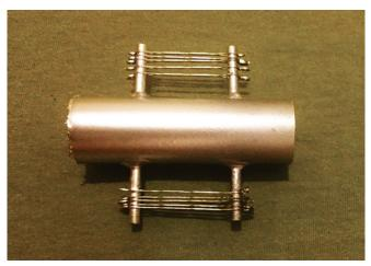
**Fig. 1:** Custom jig for stimulation of stretched elastomeric chains (four loops of closed elastomeric chain, originally 11 mm were stretched to 25 mm)
