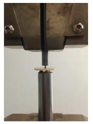
Fig. 2: Biaxial flexural strength testing using universal testing machine
