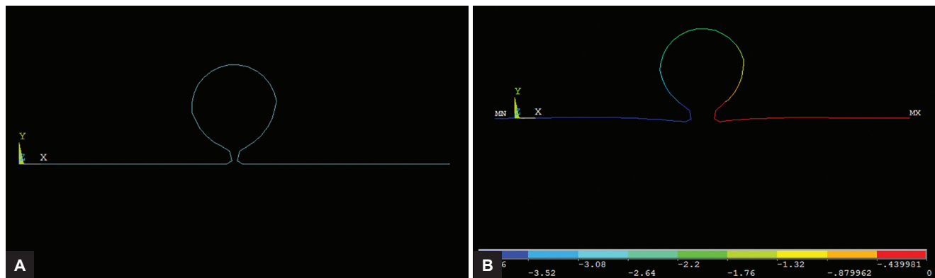
Figs 4A and B: Omega loop without preactivation bends. (A) Base model, (B) Model after 4 mm activation
