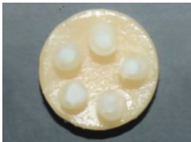
Fig. 4: The assigned resin cement was mixed and applied through the tubes to the ceramic
