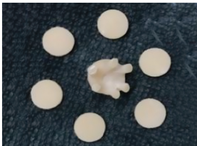
Fig. 2: Disks were removed from the ring and cut the sprue
