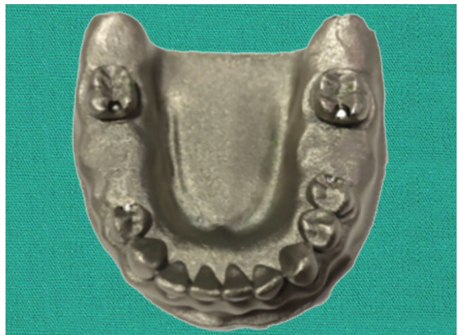
Fig. 2: A cobalt-chromium model used to evaluate the fit of all RPD frameworks
