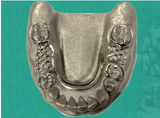
Figs 5A and B: (A) RPD framework fabricated by CLW technique seated on the reference model; (B) RPD framework fabricated by SLM technique seated on the reference model
