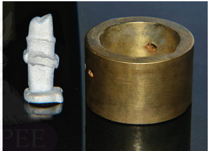
Fig. 3: Cast die and brass cylinder
