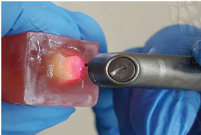
Fig. 3: Exposing to Er:YAG laser with R02-C hand piece without contact (Fotona®, LightWalker, USA)
