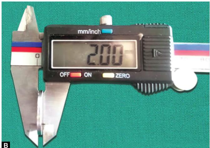
Figs 2A and B: (A) Diameter of the metallic die; (B) Thickness of the metallic die
