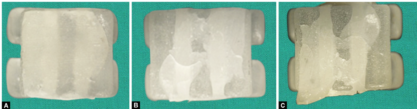
Figs 2A to C: Residual adhesive on the bracket. Adhesive remnant index scores represented as: (A) Score 1; (B) Score 2; (C) Score 3
