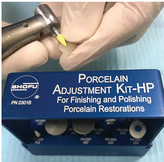
Fig. 2: Polishing the sample disk with ceramic finishing and polishing kit
