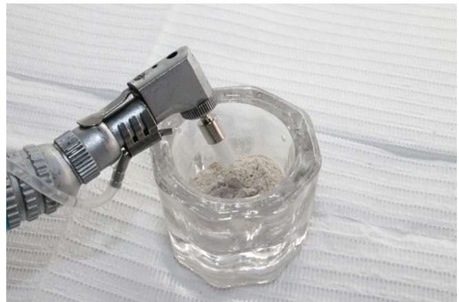
Fig. 2: Polished specimens with pumice stone
