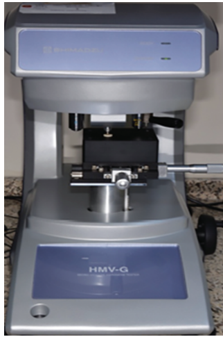
Fig. 3: Microhardness measured using a Vickers diamond indenter
