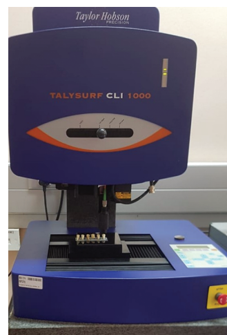
Fig. 5: Surface loss measured using profilometer
