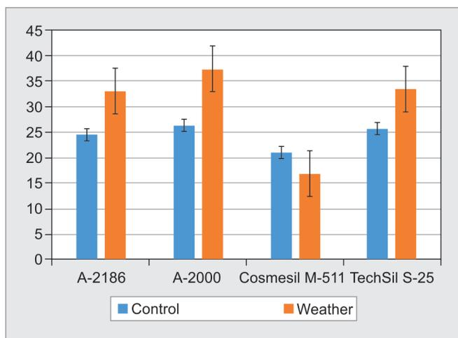
Fig. 1: Comparison between hardness of different studied materials in both weathered and nonweathered
