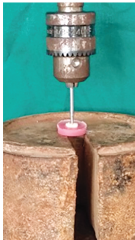
Fig. 1: Loading of the sealer with a 2-mm-diameter cylindrical stainless-steel plunger. Loading was performed on a universal testing machine
