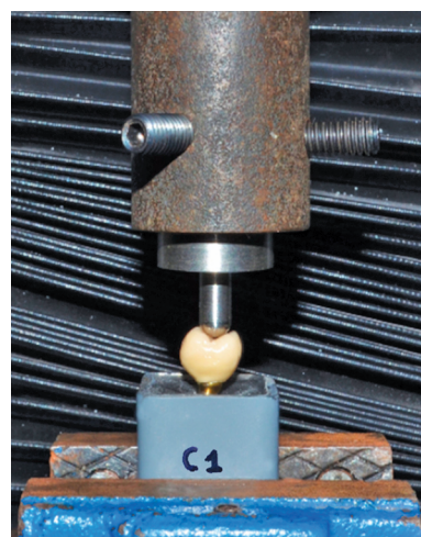
Fig. 3: Experimental set-up for fracture resistance testing
