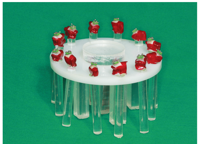
Fig. 1: Tooth specimens affixed to Plexiglas rods and glued to a Plexiglas base
