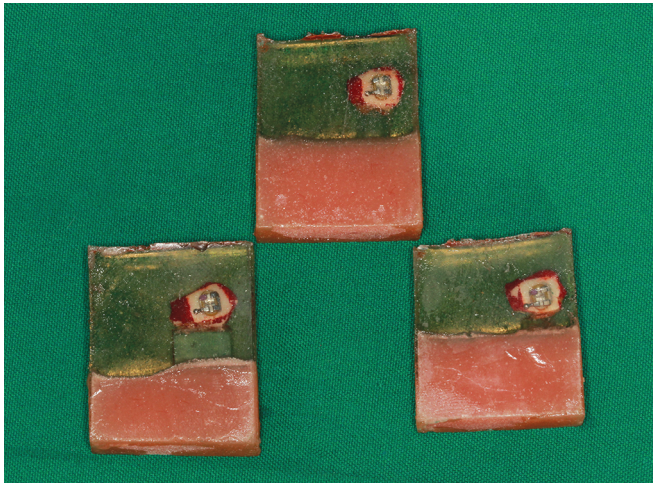
Fig. 2: Tooth specimens embedded in epoxy resin molds prior to sectioning
