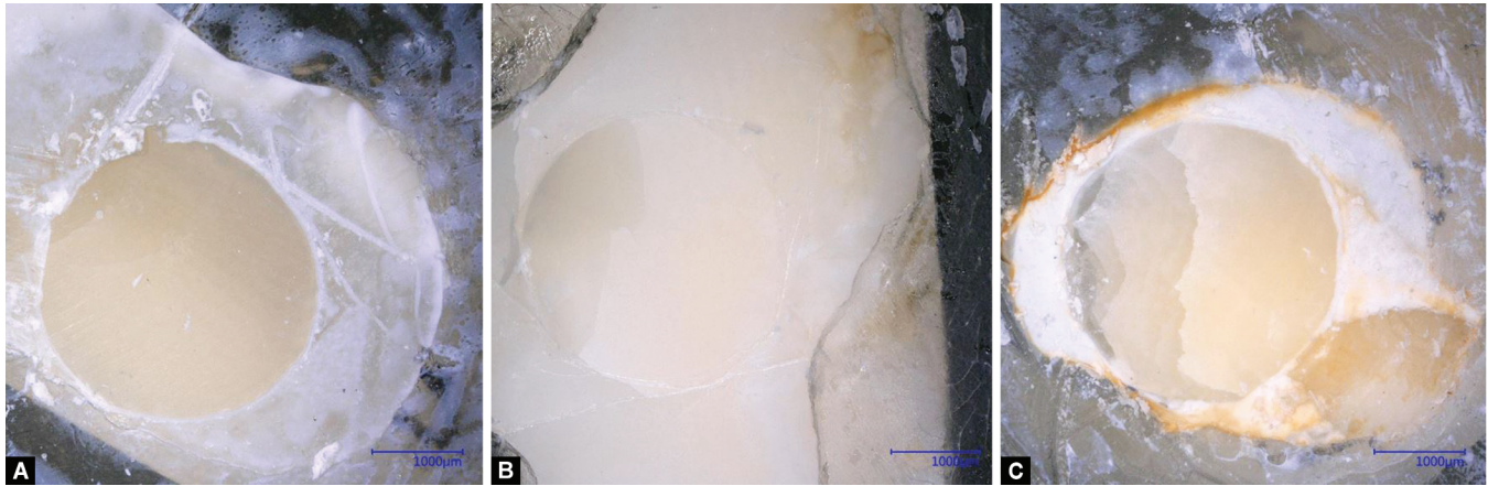
Figs 1A to C: Representative photos of numeric optical microscope of: (A) Adhesive failure ( \times 50 magnification); (B) Mixed interfacial failure ( \times 50 magnification); (C) Cohesive failure in composite layers ( \times 50 magnification)
