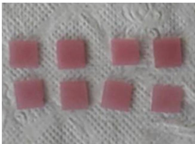
Fig. 2: Finished and polished heat-polymerized acrylic resin samples
