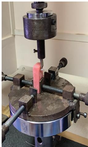
Fig. 1: Shear bond testing
