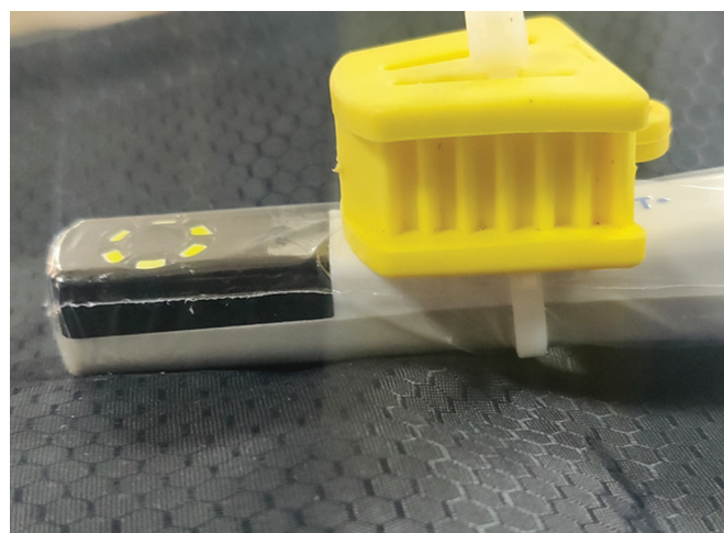
Fig. 1: Intraoral camera-bite block assembly
