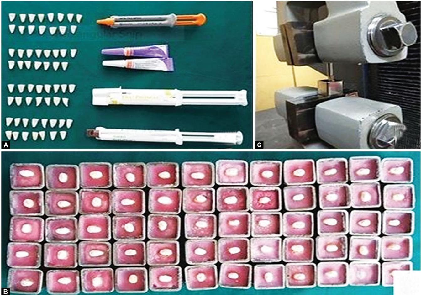
**Figs 2A to C:** (A) Sample grouping based on sealer used; (B) Tooth embedded in acrylic blocks using metal molds; (C) Fracture resistance of sample tested using universal testing machine
