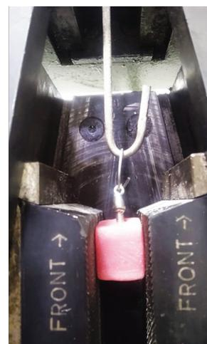
**Fig. 3:** Instron universal testing machine with sample (pull out test)
