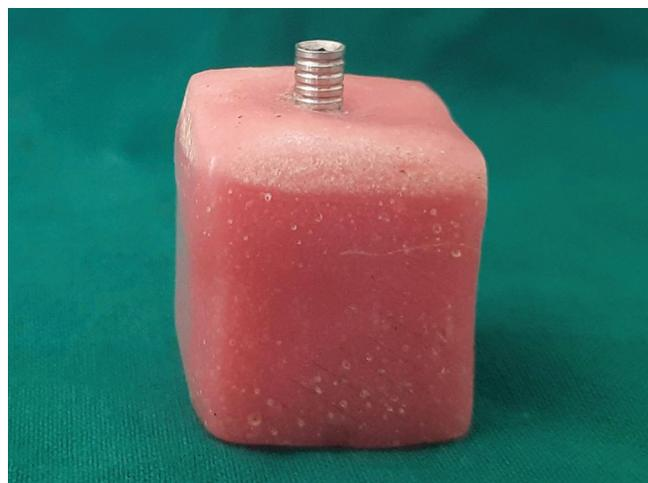
Fig. 1: Implant analog embedded in acrylic block
