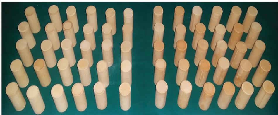
Fig. 1: Specimens for testing compressive strength
