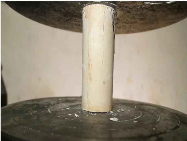
Fig. 3: Specimens for testing the compressive strength placed vertically and crushed at 1.0 mm/minute
