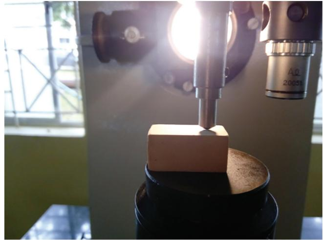
Fig. 4: Indentations made on the specimens with the indenter to test the surface hardness
