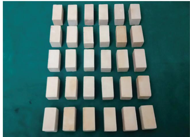
Fig. 2: Specimens for testing surface hardness
