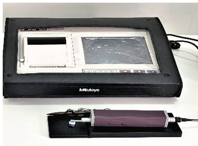
Fig. 3: Noncontact stylus profilometer used for assessing surface roughness
