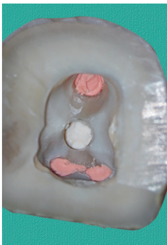
Fig. 3: Example of material dislodgement after being subjected to pushout bond test
