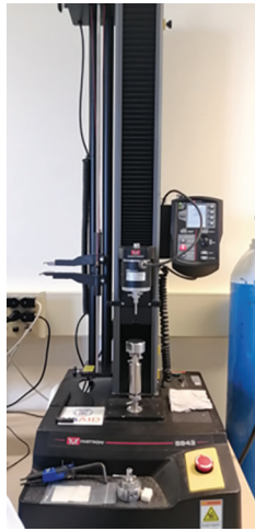
Fig. 1: The UTM (Instron 5943; Instron, Norwood, Massachusetts, USA) used to compare the fracture resistance
