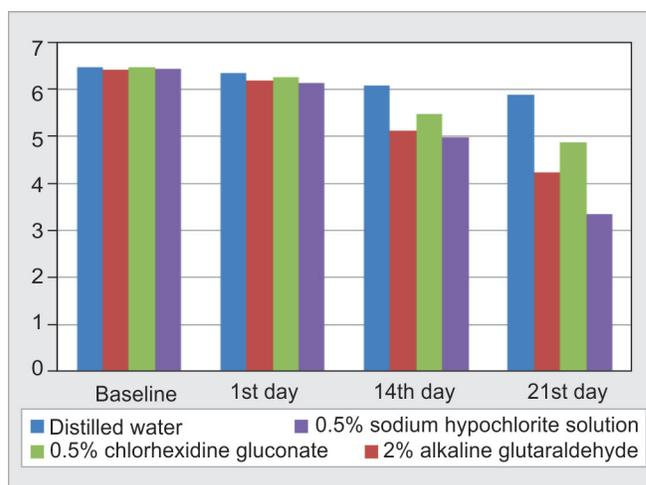
**Fig. 2:** Color stability of ProBase Hot heat cure denture base resins after immersed in the different disinfectants
