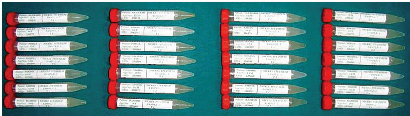
Fig. 1: Polypropylene test tubes containing CuNiTi wire samples
