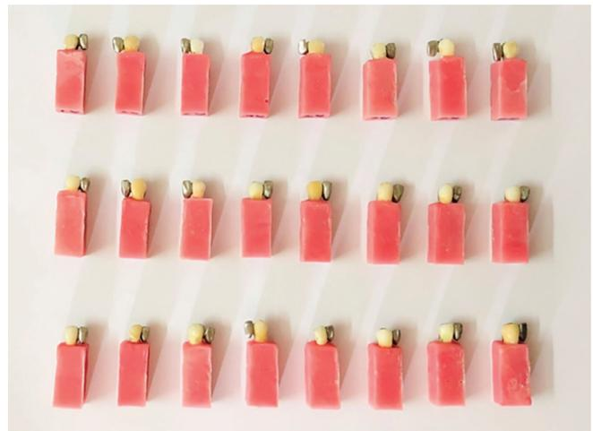
Fig. 2: Cemented prosthesis of all samples of three groups comprising cantilever design with mesh, perforated and combination of mesh and perforated design
