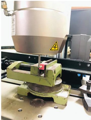
Fig. 3: Load applied on the mid-labial of pontic of the test specimen to test bond strength
