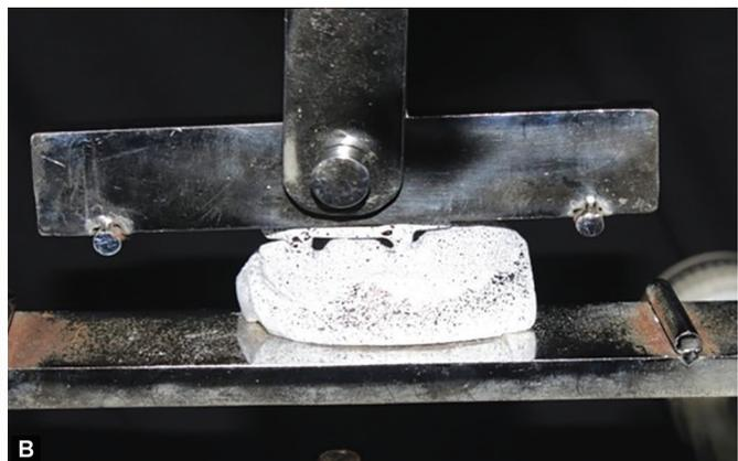
Figs 3A and B: Load applied on maxillary model. (A) Locator; and (B) Bar and clip
