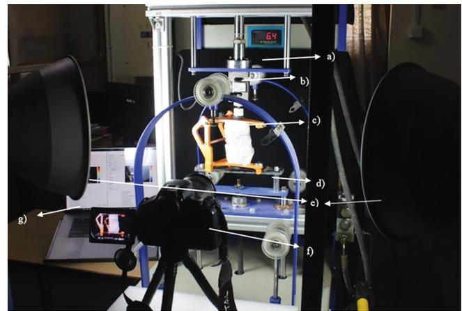
Fig. 2: DIC setup: (a) hydraulic loading; (b) load cell; (c) mounted articulator; (d) supports; (e) white light source; (f) camera; and (g) data acquisition setup
