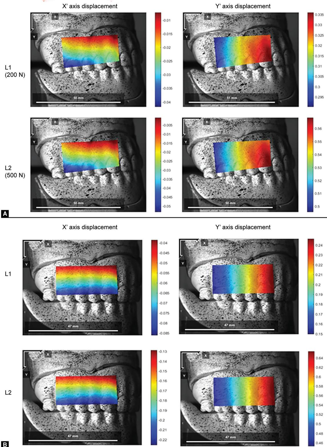
**Figs 4A and B:** Denture displacement. (A) Locator; and (B) Bar and clip
