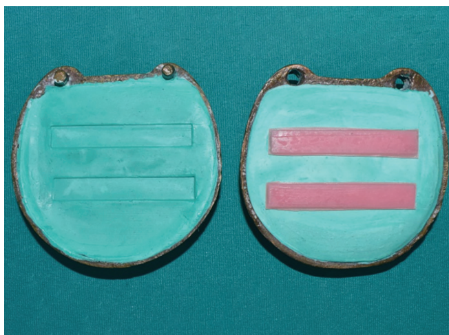
Fig. 2: Acrylized sample of dimension 60 mm length × 7 mm width × 4 mm thickness
