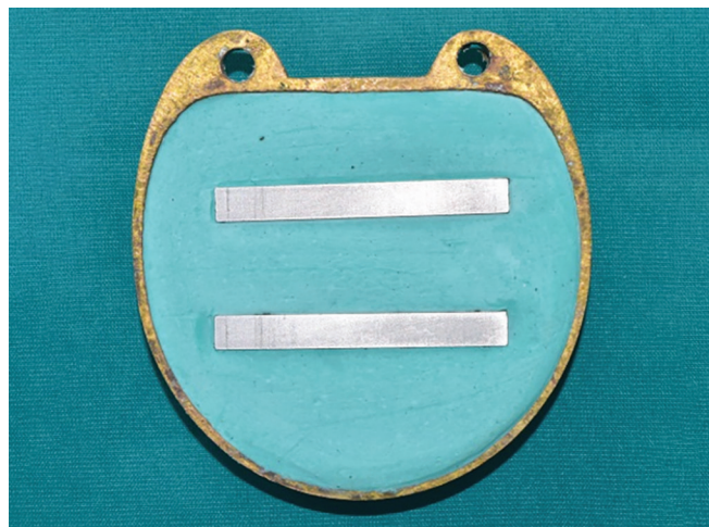
Fig. 1: Stainless steel dies invested in a flask
