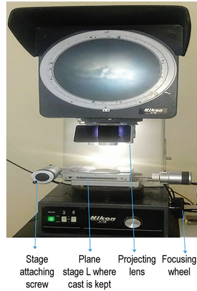
Fig. 3: Profile projector (NikonV-12A) used in the present study
