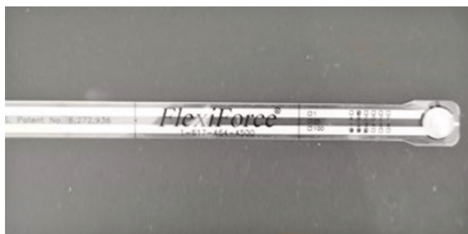
Fig. 2: Circular measurement sensor with 0.375 cm diameter
