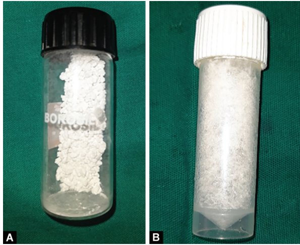
Figs 1A and B: (A) The prepared calcium phosphate cement graft for the control group; (B) The prepared polymer microspheres
