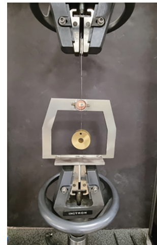
Fig. 1: Demonstration of the sliding test using Instron universal testing machine
