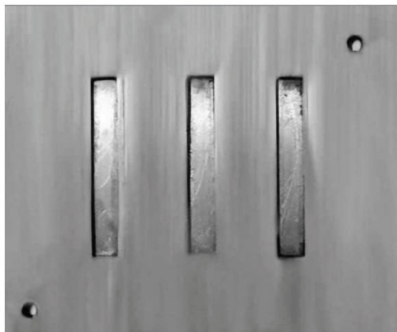
Fig. 3: Split brass mold measuring 65 mm in length, 10 mm in width, and 2.5 mm in thickness was used
