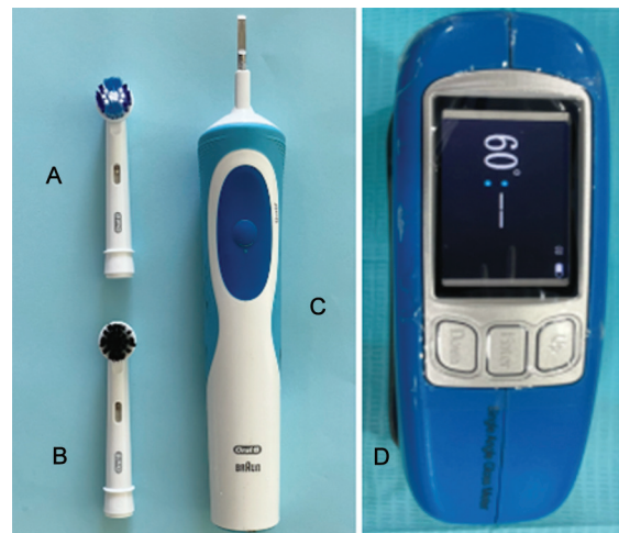
Figs 2A to D: Clinical images of the devices utilized in the study. (A) The standard toothbrush replacement head; (B) The charcoal-infused toothbrush replacement head; (C) The electric toothbrush; and (D) The gloss meter
