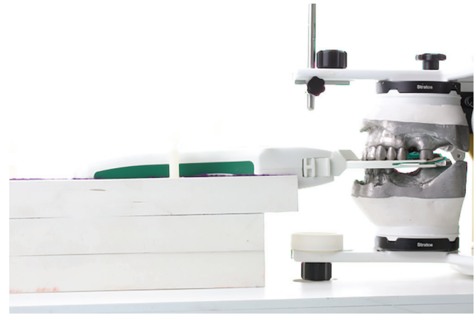
Fig. 1: T-scan device positioned in the positional jig and recording the contacts in MIP
