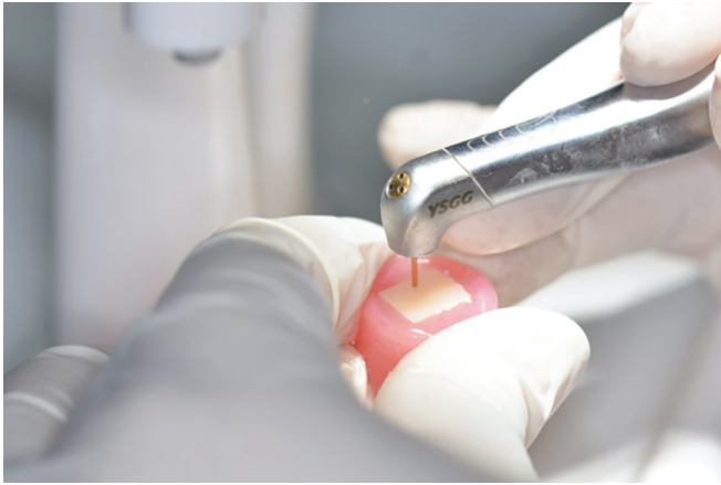
Fig. 1: Zirconia roughening by Er:Cr:YSGG laser
