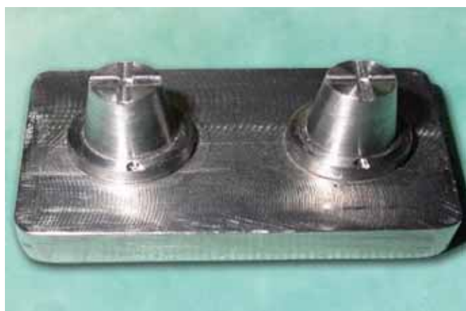
Fig. 1: Master stainless steel model containing two shouldered full crown preparation (base diameter 15 mm, height from shoulder margin 12 mm, shoulder width 2 mm, taper 7°).
