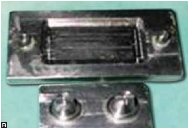
Figs 2A to D: A custom-made stainless steel tray to accommodate the master model. (A) Perforated stainless steel custom tray cover with seating channels, (B) base of the tray with locating projections and the master model adjacent to it, (C) master model in the base of the tray and (D) the tray cover over the assembly of the base and the master model
