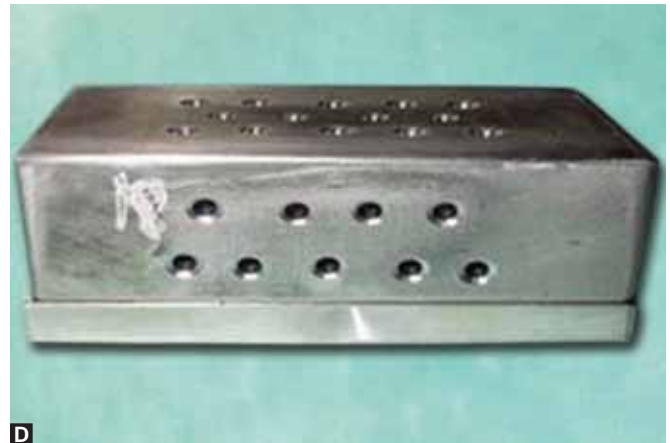
Figs 2A to D: A custom-made stainless steel tray to accommodate the master model. (A) Perforated stainless steel custom tray cover with seating channels, (B) base of the tray with locating projections and the master model adjacent to it, (C) master model in the base of the tray and (D) the tray cover over the assembly of the base and the master model
