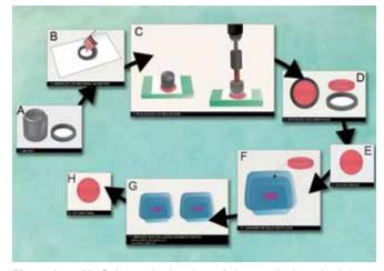
**Figs 1A to H:** Schematic drawing of the applied methodology. (A) matrix; (B) insertion of the material in the matrix; (C) impression; (D) obtaining of samples; (E) initial reading; (F) rinsing in distilled water; (G) immersion in disinfectant solution; (H) final reading
