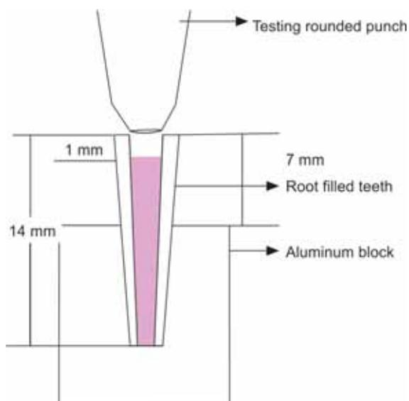
Fig. 2: Depicting fracture testing of the specimens
