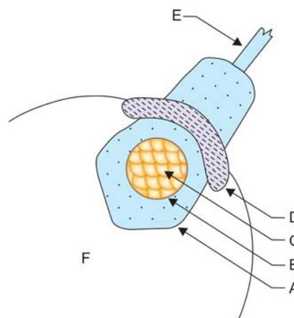
**Fig. 1:** Schematic representation of the dynamic model: (A) Nail varnish painted tooth, (B) standardized 6 mm diameter window for color measurement and bleaching, (C) bleaching material, (D) resin barrier, (E) hamilton syringe for retrieval and replenishment of acetate buffer, (F) polyvinyl siloxane jig
