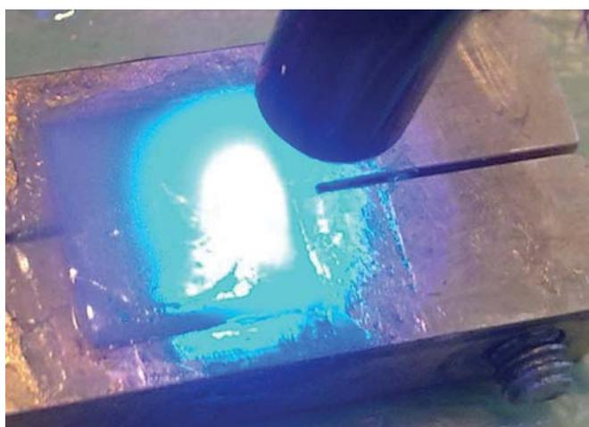
**Fig. 1:** Each 1 mm thick sampled was cured in five different poles: right upper, right lower, left lower (as shown in this figure), left upper and central zone
