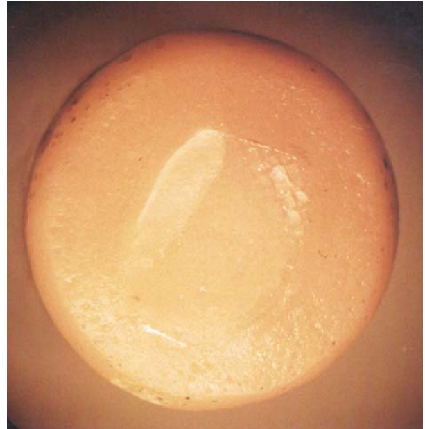
Fig. 4: Stereomicroscope view of ceramic surface (after debonding)
