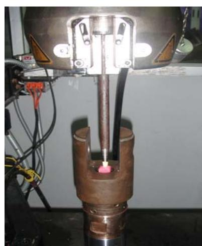
Fig. 8: The loading fixture with the specimen (Universal testing machine)
