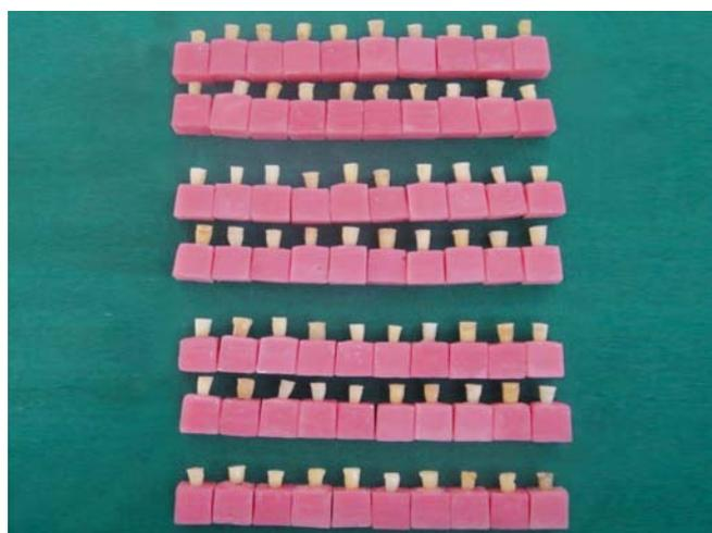
Fig. 7: Teeth embedded in acrylic resin
