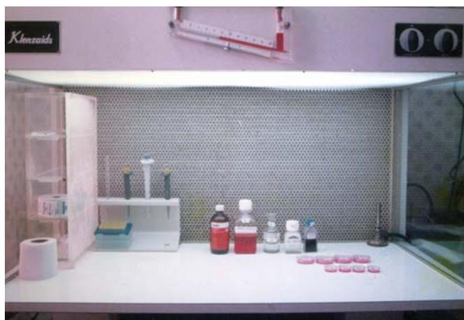
Fig. 1: Klenzaid's working bench with laminar flow of sterile air
