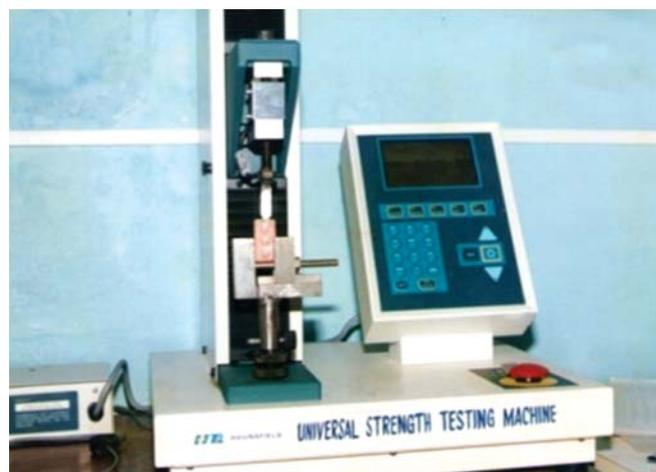
**Fig. 5:** Specimen being loaded
