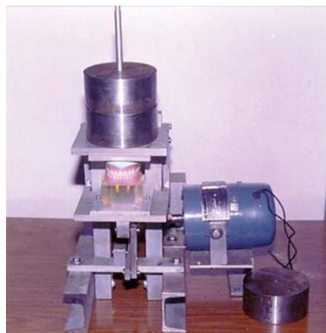
Fig. 2: Jaw simulator with dentures
