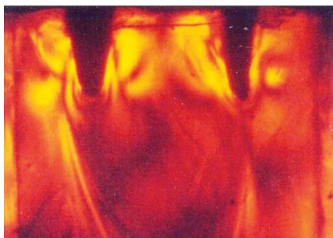
Fig. 5: Stress fringes in bar-clip at 50 lbs
