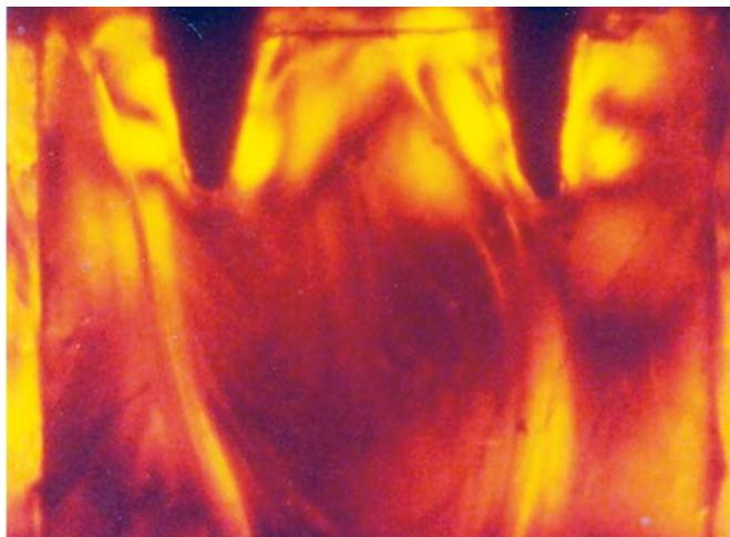
Fig. 4: Stress fringes in bar-clip at 45 lbs
