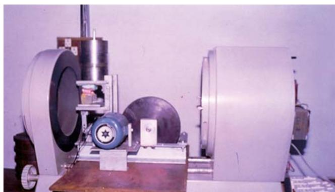
Fig. 3: Jaw simulator with polariscope
